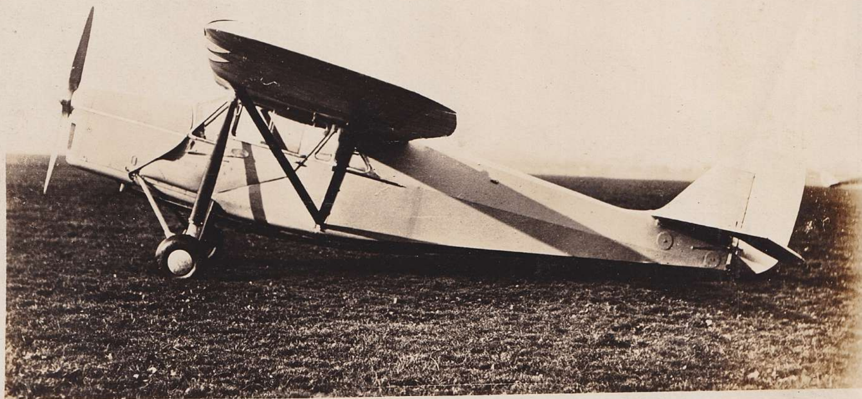
THE 1931 MODEL OF THE PUSS MOTH 120 H.P. INVERTED TYPE GIPSY III ENGINE
